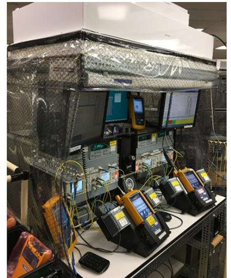
*Figure 2 - Fiber calibration station. Note the plastic around the station on the filtration system on top to reduce dust. Some of the commercially available products used are modified by Fluke Networks to meet our accuracy requirements.*
