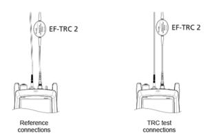
Figure 3. Reference and TRC Test Connections for Smart Remote Mode
