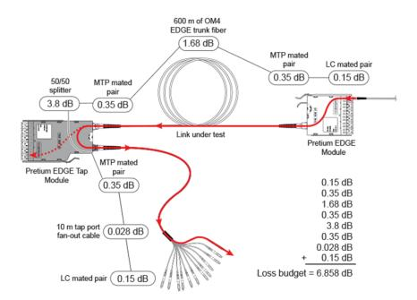
Figure 2. Example of a Loss Budget Calculation for Testing Network Links
