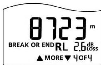
The result loss of the fiber (RL) is 2.6 dB.
