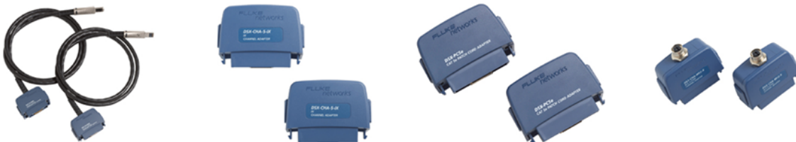
Testing different configurations of Ethernet connections requires the use of the correct adapters. Shown: Permanent Link, Channel, Patch Cord, and M12 adapters
