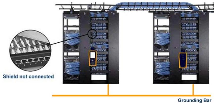
Figure 1 – Screen path through building ground
