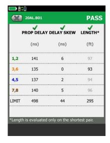
The DSX Series CableAnalyzers measure Delay Skew as part of their range of length measurements.
