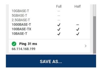
Figure 7. The LinkIQ tester displays the switch's name, its advertised speed, the specific port number and virtual LAN (VLAN) assigned to a link, and performs an IP ping test.
