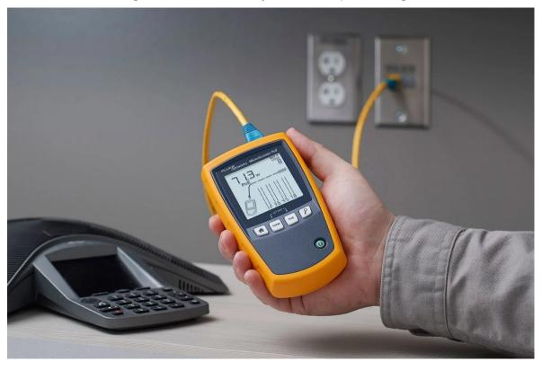
Figure 5. The Ethernet Alliance PoE-certified MicroScanner Cable Verifier displays the wattage and class (0-8 of power available on the link and indicates which pairs are carrying power.
