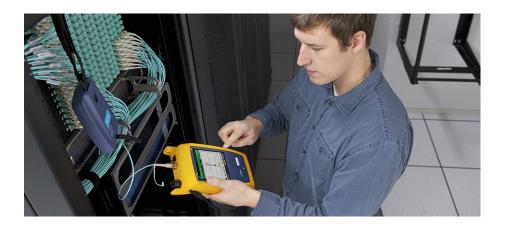
As fiber deployments become commonplace, network owners and technicians are paying more attention to the two crucial devices for testing fiber optical cables: the Optical Loss Test Set (OLTS) and the Optical Time Domain Reflectometer (OTDR).
