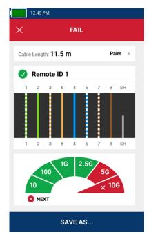
Cable test with remote attached shows remote ID number 1, length and pairing of each wire and cable performance of up to 2.5 Gb/s but failed the test due to a user-set limit of 10 Gb/s performance.
