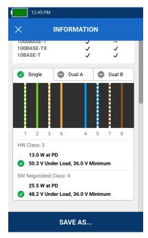
Switch port Power over Ethernet settings shows pairs used, power and class available and results of the PoE test under load.
