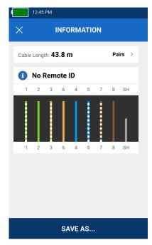
Cable test without remote attached shows length and pairing of each wire
