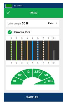
Cable test with remote attached shows remote ID number 5, length and pairing of each wire and cable performance of up to 10 Gb/s
