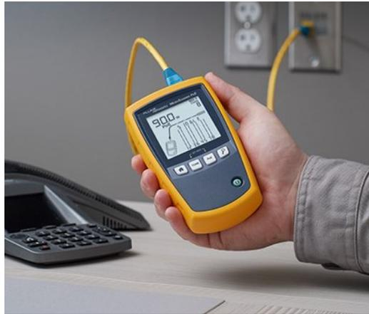
*Figure 5. The MicroScanner PoE is Ethernet Alliance Gen2 PoE certified and can detect the power offered by the PSE plus the network's speed, and features a suite of cable testing features.*
