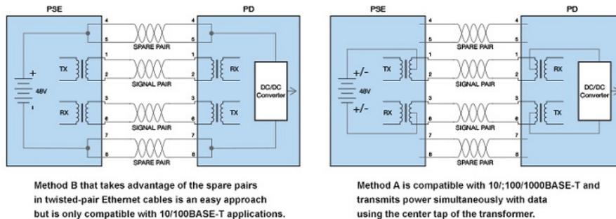
With IEEE 802.3bt, we move to a 4 pair based system to deliver the required power. We still have our PSE and PD devices, with the current flow now shared among the four pairs.
