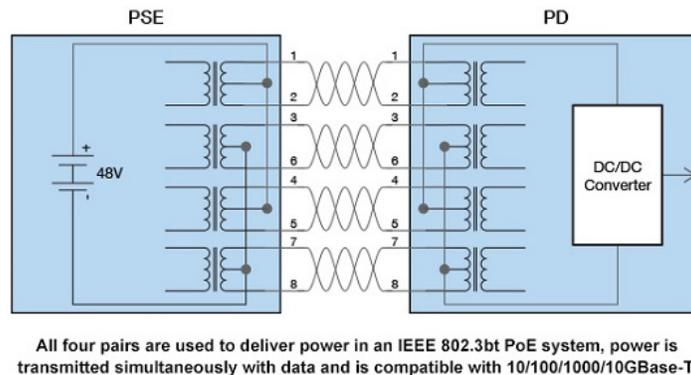
While devices can tolerate some DC resistance unbalance, too much unbalance causes the potential for saturation of the transformer. This can ultimately distort the waveform of Ethernet data signals, causing bit errors, retransmits and even non-functioning data links. With a four pair PoE system some DC resistance unbalance between the pairs can be tolerated, but if it is excessive, PoE will stop functioning.
