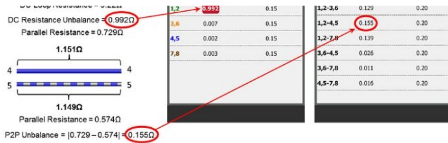
Figure 1 While not required in field testing, the DSX-5000 CableAnalyzer can be configured to include DC Resistance Unbalance test limits for either Channel or Permanent Link Measurements; as shown in Table 1 below.
