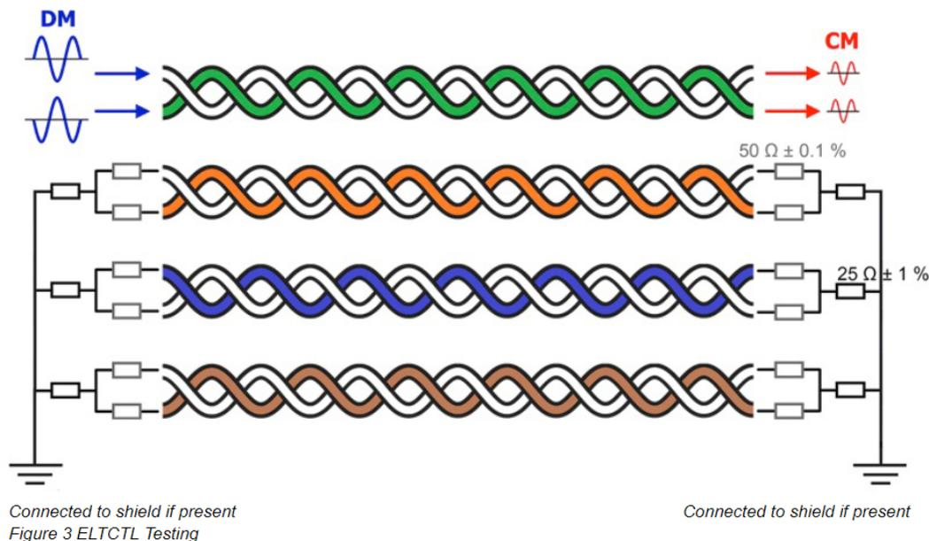
While TCL and ELTCTL parameters are excellent indicators of the balance of a twisted-pair cable, neither is currently a field test requirement under ANTI/TIA-568.C.2 standards. This is because most field test equipment has only been capable of differential mode measurements. TCL and ELTCTL testing have therefore been limited to laboratory environments by manufacturers who must ensure good pair balance characteristics to comply with TIA and ISO/IEC industry performance standards.
