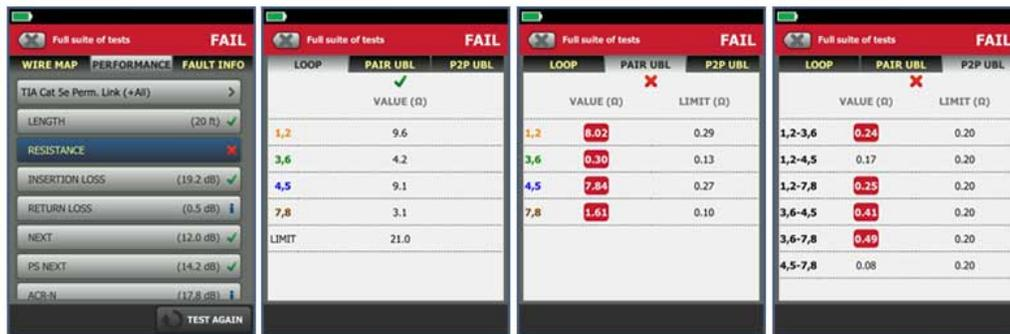
The field testing standard for ANSI/TIA 1152 now includes DC Resistance Unbalance as a field test. Limits are included in ANSI/TIA-568-C.2. It is not a mandatory certification requirement, it is easy to include if you have a capable cable tester like the DSX-CableAnalyzer. But there's a catch. While ISO/IEC 11801 ed. 2.2 provides DC Resistance Unbalance test limits for the Channel and Permanent Link definitions, ANSI/TIA-568-C.2 only provides test limits for the Channel definition.
